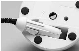
Slide the connection plug of the power pack into the socket on the underside of the charging base. Tilt it slightly and apply slight pressure until you hear and feel it snap into place. Place the charging base on a suitable, flat table top.
