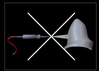
Fig. 6 Sandblasting at the incorrect angle.
