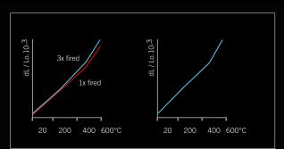
Fig. 3 Comparison of CTE increase:Unstable CTE of otherStabilised CTE ofdental ceramic afterHeraCeram Saphirmultible firing.after multiple firing.
