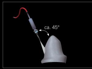
Fig. 5 Sandblasting at the correct angle.
