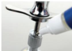
Add 1-2 drops of oil to the turning mechanism.
